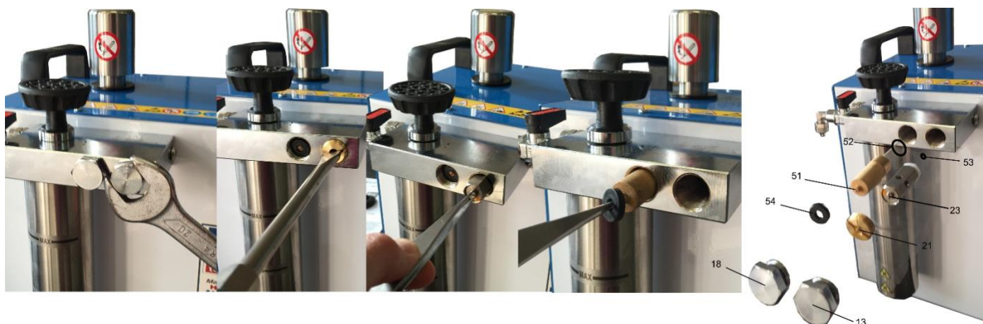
FIG 4 – CHECK VALVE AND BACK FLAME FILTER REPLACEMENT
