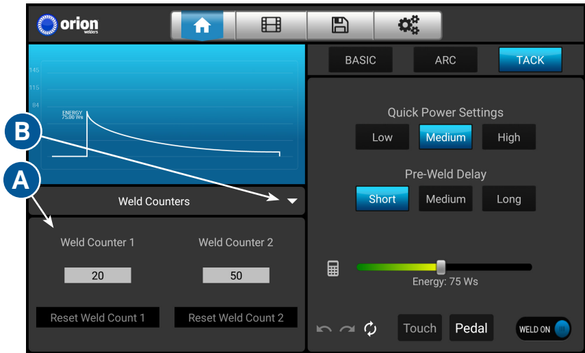
Figure 22.1. The Mini-Screen Area (A) displays additional information. You can customize what information you wish to view. Touch the down-arrow button to view a list of available information widgets.
