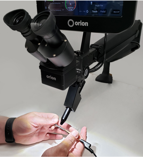
Figure 13.1. Rest your hands on the table and position the workpiece close to, but not touching the electrode. Then look through the microscope.
