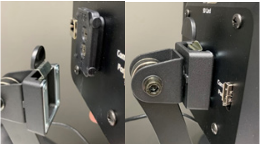
Figure 4.1. Attach the Touchscreen to the Microscope Arm Assembly. Remove the screen protector film.
