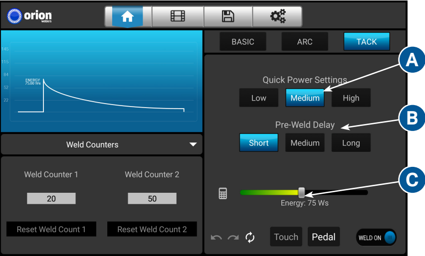
Figure 20.1. The Parameter Selection Area with the Tack layout selected.
