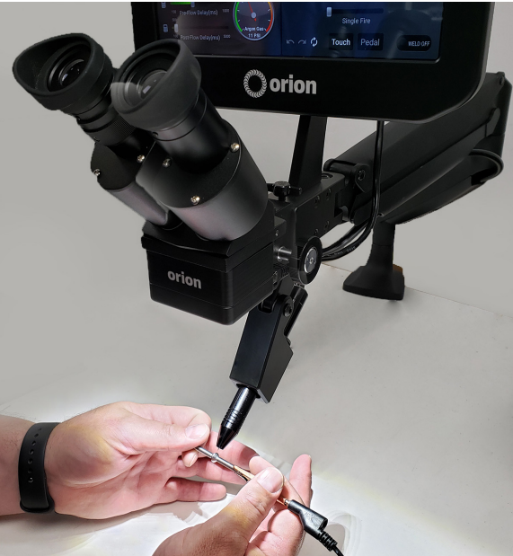
Figure 34.1. Adjust the arm to a comfortable height. Ideally your hands will be able to rest on the table while making welds for greatest stability.
