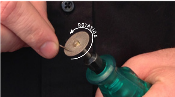
Figure 9.1. A sharp electrode tip improves arc initiation and results in a better overall weld.
