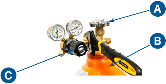
Figure 12.1. First, turn the regulator dial (C) counterclockwise to close the regulator valve. Screw the gas regulator (A) to the top of the shielding gas tank (B).
