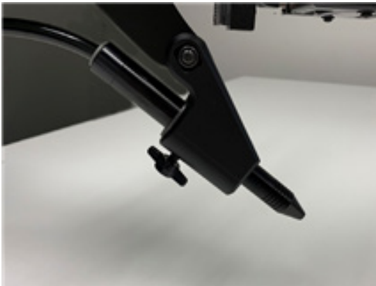
Figure 5.1. Mount the Welding Stylus to the holder below the microscope.
