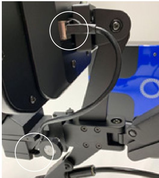
Figure 4.3 After installing the rubber eyepiece covers, use the Shutter Cable to connect the Touchscreen to the bottom of the microscope head.
