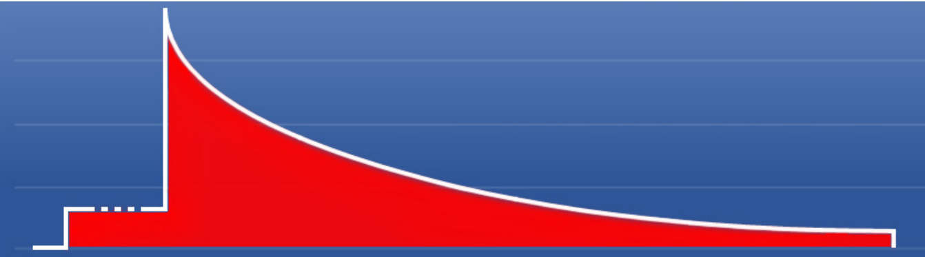
Figure 38.1. The red area illustrates the total amount of energy released during a weld.
