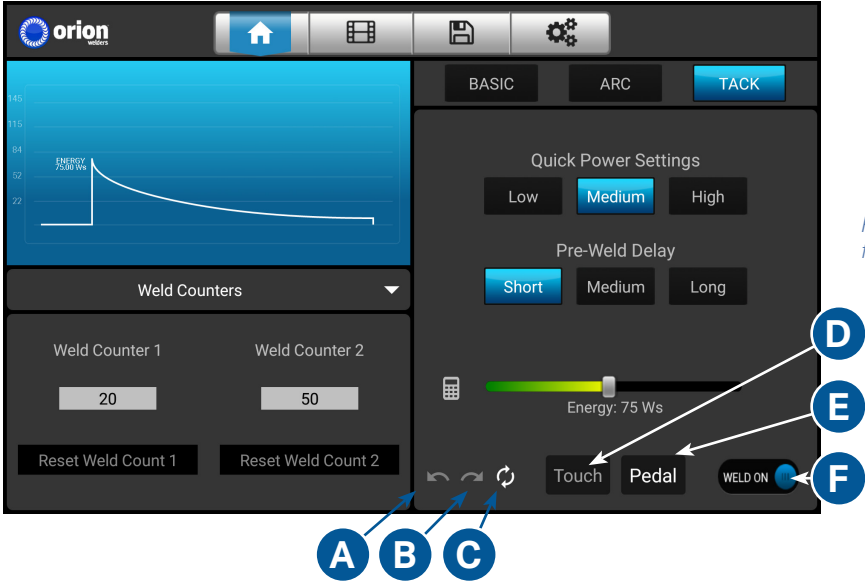
Figure 21.1. The Footer buttons display at all times for convenient access.
