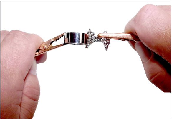
Figure 35.2. In Tack Mode, you'll use two different alligator clips to hold two different work pieces. Touch the two pieces together where you wish to place a tack weld, thus tacking one work piece to another.
